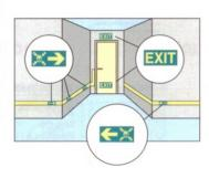
2. The LLL shall be installed at the door frame or at the door leaf up to the exit door handle.
