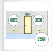
1. In all corridors, the visual effect of the LLL system shall be continuous, except where interrupted by intersections with other corridors, cabin door or local enlargement, to provide a visible delineation along the escape routes.
