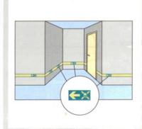
5. In dead-end corridors, the LLL system shall include arrows or equivalent direction indicators, at intervals of no more than 1 m, pointing away from the dead end.
