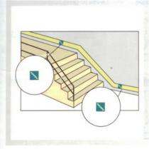
3. In all stairways on the escape route, LLL installed on the bulkhead shall be at a height no more than 300 mm above the forward edge of each step. The top and the bottom of each set of stairs shall be identified to show that there are no further steps.
