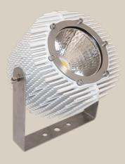
The LED floodlights are designed for a long lifetime and high efficiency. The LED gives instant light and is immune against voltage drops. The special design of seawater resistant aluminium anodized module housing secures an excellent cooling. Mounting frame and bracket are made of stainless steel.
